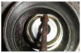
11. Install a new OEM Mazda dust cap per normal procedure. The new bearing cartridge has a metal dust "shield" on the outboard side of the cartridge, but it is not a watertight rubber seal like what's used on the inboard side. It is important to continue using the OEM dust cap to stop water and debris from entering the bearing.
