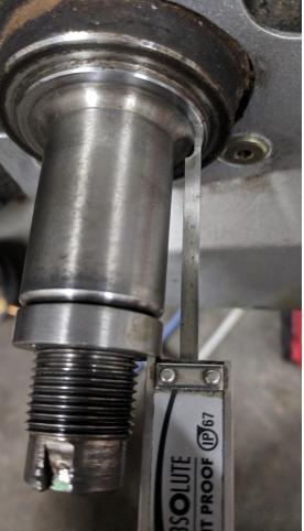
7. Slide the adapter sleeve over the spindle and threaded support ring. Since you likely won't have to touch these for quite a while! apply a thin layer of anti-seize or high temp grease on the spindle to help later removal/servicing. The sleeve can be tight, just make sure it's straight and install it over the support ring. You may need to use some fine grit emery cloth on the threaded ring to get the sleeve to slide over it. If it seems too tight please contact us, do not force it on.
