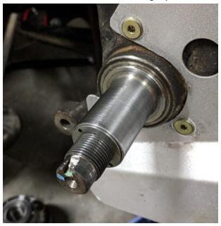
8. Install the pre-assembled hub unit onto the spindle over the adapter sleeve, ensure the inner races are straight and do not force it on. Align the bearing and it will slide on and fully seat all the way on to the end of the spindle similar to stock.
